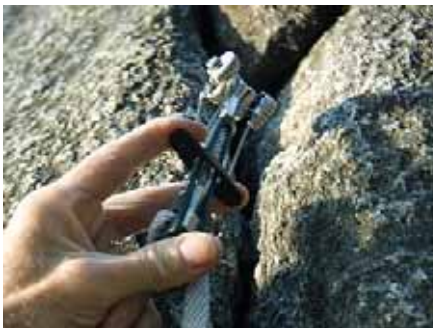
Spring-loaded Cam for Protection
